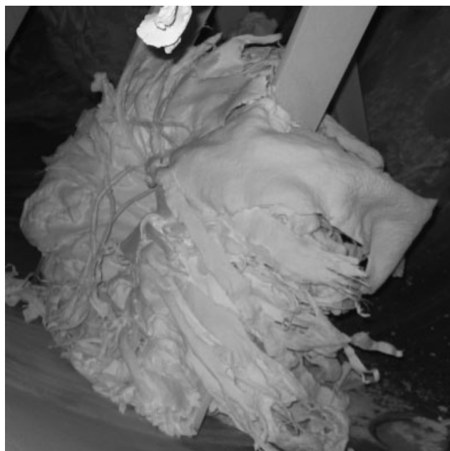
Figure 3. Type two: serious “floculent sheets” occupied the head of the paddles.
