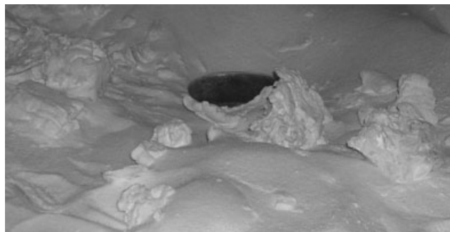
Figure 1. Type one: “spherical lumps” formed by hot spots in an industrial HSBR.
